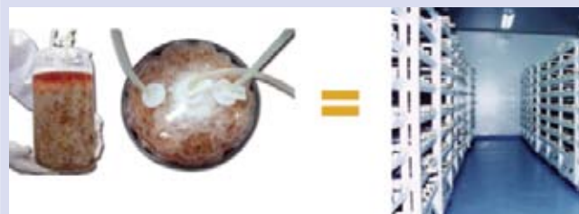
Figure 7: Cell biomass from a single, 5-L Current perfusion bioreactor (with 150 gram paper carrier) equals that of 150 roller bottles for vaccine production cell culture.
