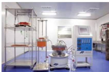
Photo 1: 5-L Current perfusion bioreactor system
