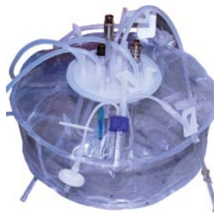
Photo 3: Disposable 5-L plastic bioreactor bag with DO, pH, and temperature probes
